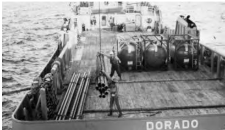
Figure 4.6. Deckhands loading drill pipe onto a supply vessel
